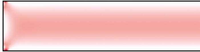
Figure 17. Intensity contour plot of \sigma_{xy} given by the 64 \times 16 OPT mesh. Stress node values averaged between adjacent elements. The root singularity pattern is visible.
